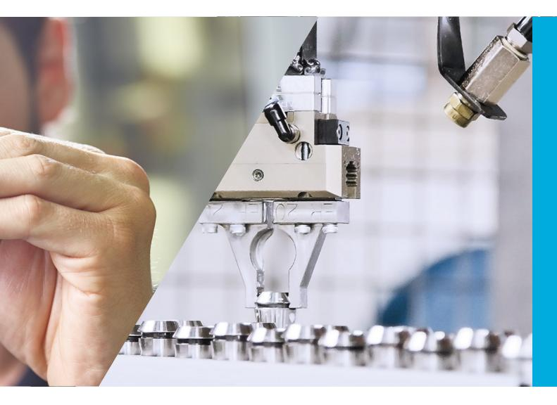
Rely on the original Outstanding design paired with experienced engineering make our ER products one of the most successful toolholding options worldwide. Our ER clamping collets exceed the DIN requirements and convince with a solid collet TIR of up to  $5\,\mu m$ .
