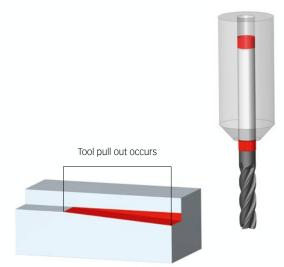
Changes in length can cause damages to the workpiece.
