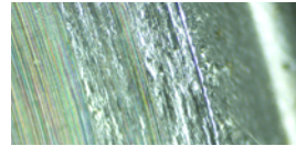
Bare metallic clamping nut after 15 clamping cycles
