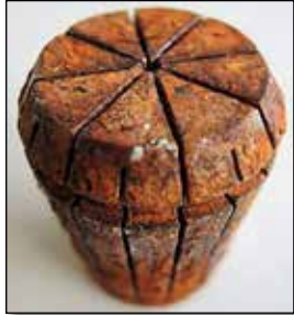
Standard ER Collet / Material: Conventional Spring Steel
