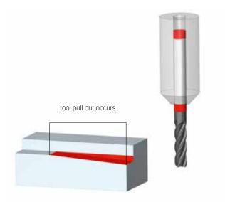
Changes in length can cause damages to the workpiece
