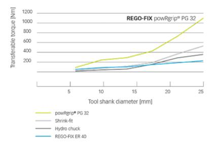
Measured transferable torque per shank diameter / Source: In-house testing
