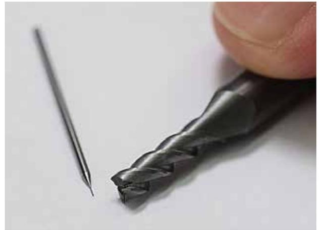
Low-stress aluminium (closeup with micro tool). Machining tool with 0.15 mm diameter.
