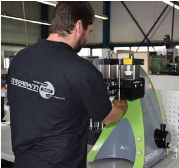
powRgrip system: A unique tool clamping system that clamps tools in seconds at the touch of a button and without heating, and that also has a sustainably precise concentricity even for the smallest tool diameters.
